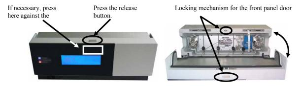
Fig. 13: Tilting the front panel downward
