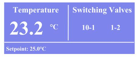
Fig. 25: Front panel display (here: for an FLM with two 2-position/10-port switching valves)
