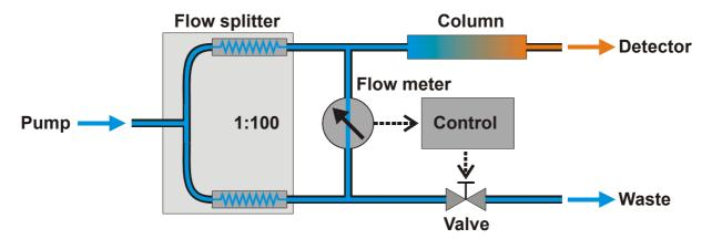
Fig. 1: Operation principle of flow splitting with control
