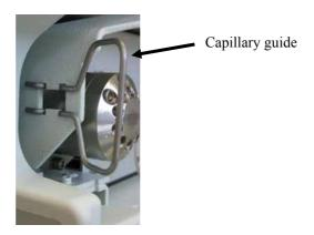
Fig. 19: Capillary guide installed on the carrier
