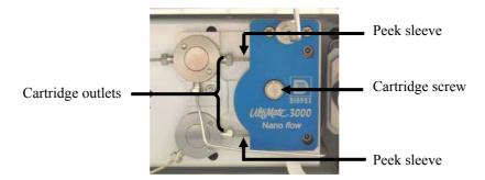
Fig. 23: Splitter cartridge
