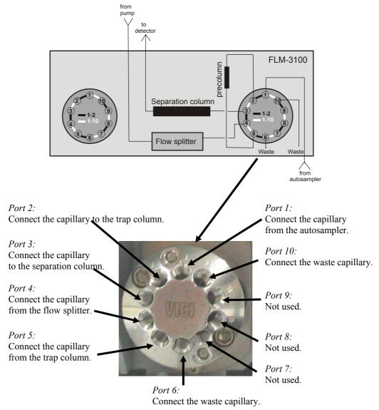
Fig. 21: Example for the connections on a 2-position/10-port column switching valve
