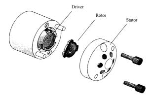
Fig. 45: Exploded view of the Valco model C2 valve
