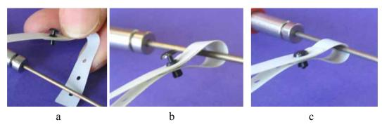
Fig. 39: Clipping the column ID chip card onto a column
