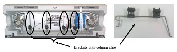
Fig. 16: Brackets with column clips
