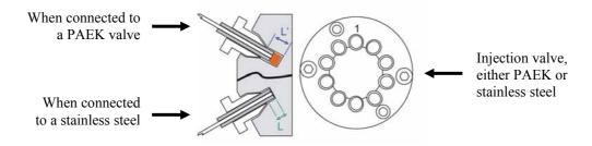
Fig. 2: Capillary connection on the injection valve
