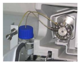
Fig. 24: Flow Manager with manual injection port
