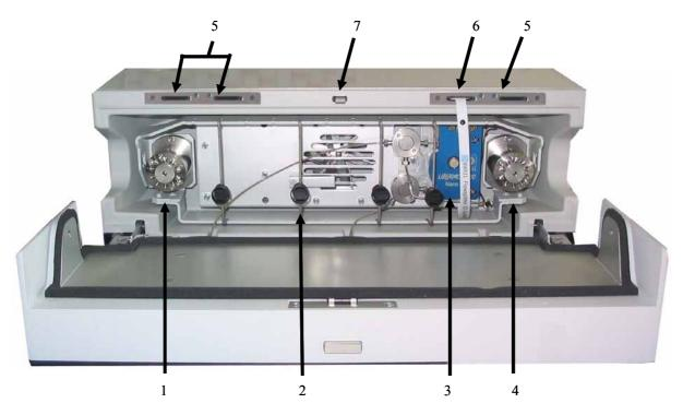
Fig. 8: Open FLM-3100 (here: with two 2-position/10-port switching valves)
